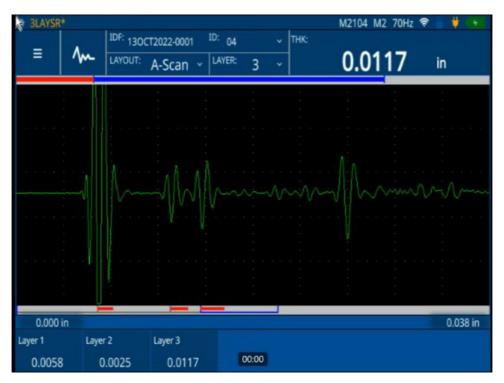
50 MHz measurement of a three-layer plastic container performed on the 72DL PLUS ultrasonic thickness gauge
